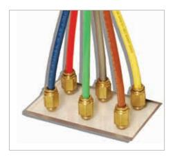
Parflex 1120 Series Tubing is developed for brake system connections that maintain a basically fixed relationship between couplings during vehicle operation. Tubing is made from nylon and is available in more than ten colors for quick identification of lines.
