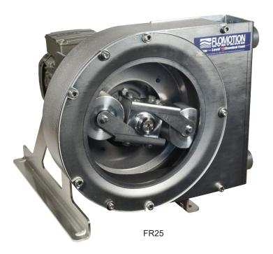
The FR25 is a two roller peristaltic pump designed to handle abrasive slurries, viscous fluids, and aggressive chemicals that are normally difficult to pump with other types of positive displacement technologies. The FR25 is an ideal choice for metering, batching and transfer applications. Peristaltic pumps are becoming the standard for hard to handle fluids such as Sodium Hypochlorite that off-gas and vapor-lock diaphragm pumps.
