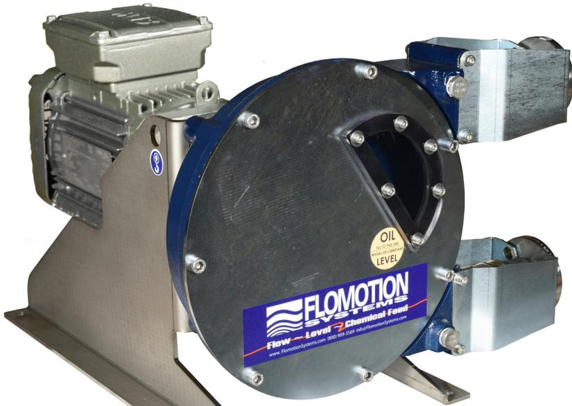
The FS25 Series peristaltic pump is a two-shoe design, 180° apart on a rotating wheel, successively compressing a reinforced rubber hose. The motion of the shoes compresses the rubber against the pump housing creating continuous suction at the inlet of the pump and pushing the fluid to the outlet of the pump.
