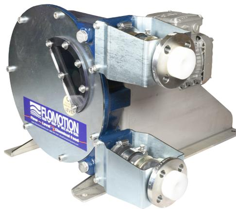
The sealed pump casing contains a lubricant that reduces friction of the shoes moving over the rubber hose. The pumped fluid is in contact only with the interior of the rubber hose, thus permitting the pumping of a wide variety of reactive fluids.
