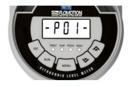
This mode is used to set up the LT330 or change information already set, this is achieved by using the 5 push buttons located either side of the display.
