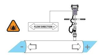
The insertion sensor must be installed correctly in relation to the liquid flow direction in the pipe. Ensure that the flow direction is known. The flow rate will be measured in the positive direction when the liquid in the pipe is flowing from – to the + direction as indicated on the tag plate of the sensor.
