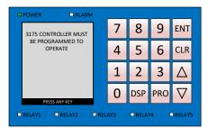
When the controller is first powered up, you should see this screen. Press any key to access the Process screen.
