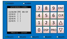
This is the Manual Override screen. Press keys 1-5 to activate/de-activate the associated relays. Verify valve and/or pump operation. The override will automatically release after 5 minutes. Press "CLR" to return to the Process Screen.
