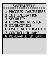
Note: Failure to follow the previous procedures could result in SD card file corruption. All data log history will be lost and the SD card will have to be replaced or re-formatted on a PC for data log writing to occur.
