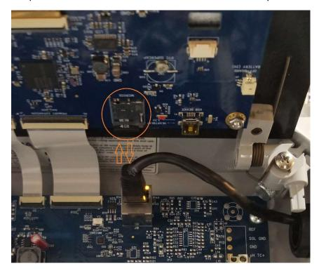
The SD card is inserted and initialized at the factory. Follow the instructions below to remove the SD card and retrieve the data log.
