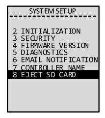
2) The micro SD card can now be removed by pressing up until the card clicks and releases from its mount.
