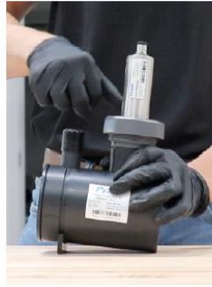
Tighten Sensor Nut
