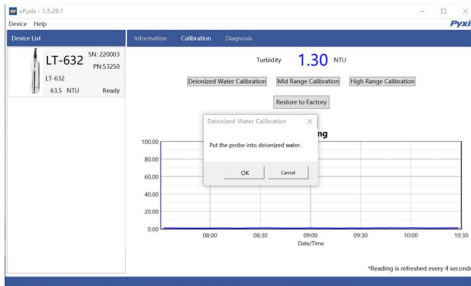
Figure 22 - Deionized Water Calibration
