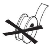
DO NOT use thread seal tape on pump tube threads.
