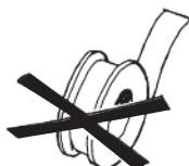
**DO NOT use thread seal tape on pump tube threads.**
